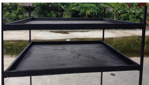
Fig. 3. Table 2 floors for drying organic fertilizer of rubber farmers has small pores for circulate the air
